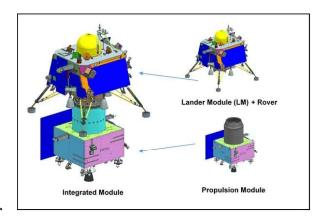
landing and maneuvering and various sensors for navigation, guidance, control, hazard detection, and touchdown. The **rover module**, **Pragyan**, can travel up to 500 meters and has two science payloads: **APXS and LIBS**. The mission is expected to last one lunar day for the lander and rover and up to six months for the propulsion module.
